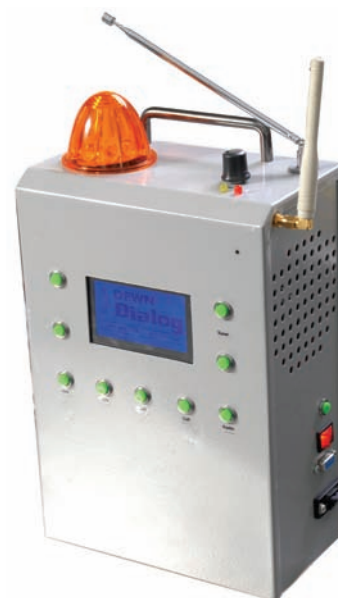
The DEWN alarm device developed by the Dialog- University of Moratuwa Mobile Communications Research Laboratory
